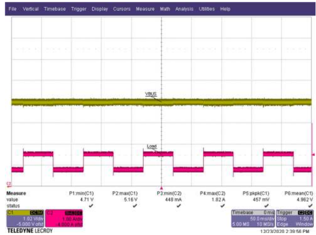
Figure 105 – Transient Response. 265 VAC, 5 V, 25% to 50% Load. V_{OUT} = 5.16\text{ V max.}, 4.71\text{ V min.} CH1: V_{OUT} , 1.02 V / div. CH2: I_{OUT} , 1 A / div. Time: 50 ms / div.
