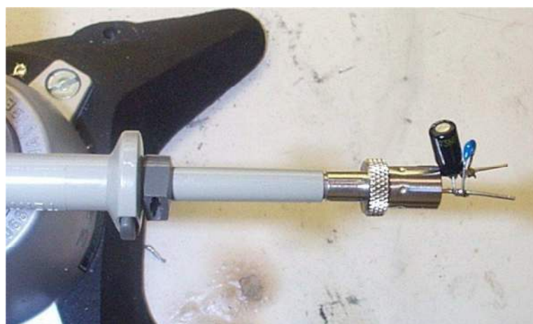
Figure 101 – Oscilloscope Probe with Probe Master ( www.probemaster.com ) 4987A BNC Adapter. (Modified with wires for ripple measurement, and two parallel decoupling capacitors added)
