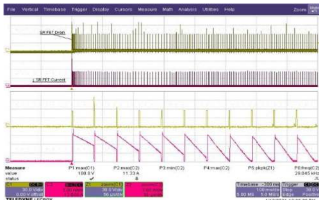
Figure 71 – SR FET Drain Voltage and Current. 265 VAC, 5.0 V, 3 A Load. V_{DS\_SRFET} = 101 V Maximum. CH1: V_{DS\_SRFET} , 30 V / div. CH2: I_{DS\_SRFET} , 3 A / div. Time: 100 ms / div. (56 \mu s / div. Zoom)
