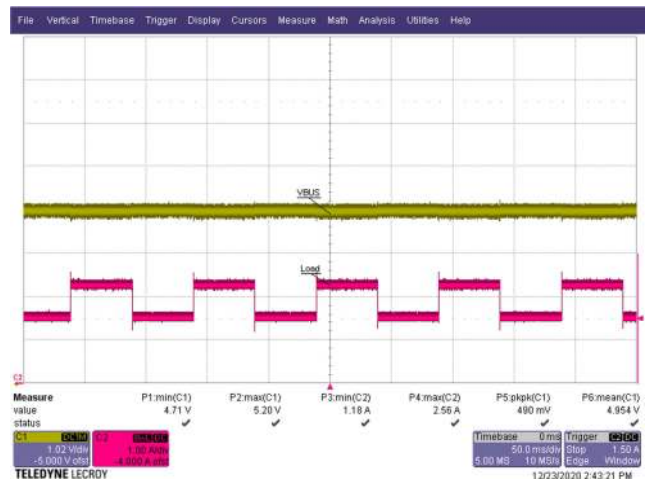
Figure 107 – Transient Response. 265 VAC, 5.0 V, 50% to 75% Load. V_{OUT} = 5.20\text{ V max.}, 4.71\text{ V min.} CH1: V_{OUT} , 1.02 V / div. CH2: I_{OUT} , 1 A / div. Time: 50 ms / div.
