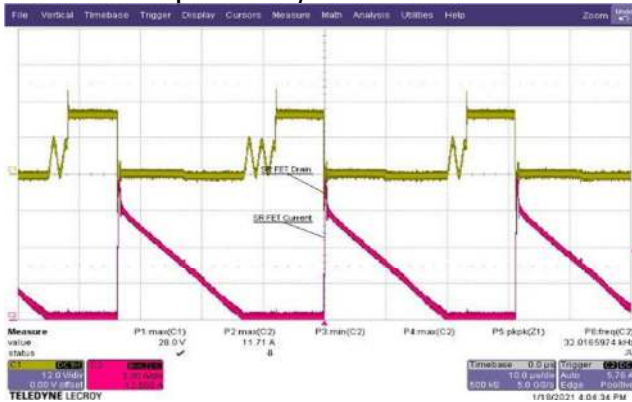
Figure 82 – SR FET Drain Voltage and Current. 90 VAC, 5.0 V, 3 A Load. V_{DS\_SRFET} = 28.0 V Maximum. CH1: V_{DS\_SRFET} , 12 V / div. CH2: I_{DS\_SRFET} , 3 A / div. Time: 10 \mu s / div.
