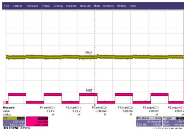
Figure 110 – Transient Response. 90 VAC, 9.0 V, 0 to 25% Load. V_{OUT} = 9.23 \text{ V max.}, 8.74 \text{ V min.} CH1: V_{OUT} , 1.02 V / div. CH2: I_{OUT} , 1 A / div. Time: 50 ms / div.
