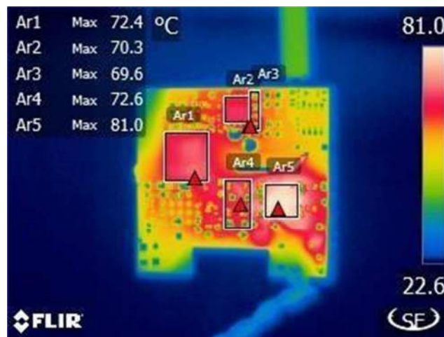
Figure 39 – Bottom Thermal Image, T_{AMB} = 22.8\text{ }^{\circ}\text{C} . Ar1: InnoSwitch3-PD, U_1 = 72.4\text{ }^{\circ}\text{C} . Ar2: SR FET, Q_2 = 70.3\text{ }^{\circ}\text{C} . Ar3: SR FET Snubber = 69.6\text{ }^{\circ}\text{C} . Ar4: Primary Snubber = 72.6\text{ }^{\circ}\text{C} . Ar5: Bridge Rectifier, BR_1 = 81.0\text{ }^{\circ}\text{C} .
