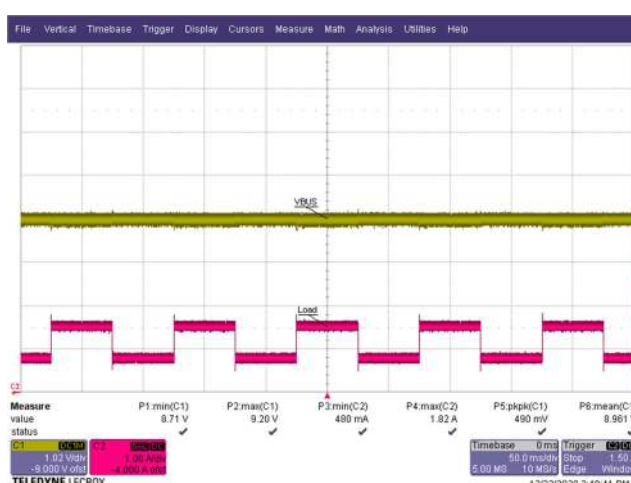
Figure 113 – Transient Response. 265 VAC, 9.0 V, 25% to 50% Load. V_{OUT} = 9.20 \text{ V max.}, 8.71 \text{ V min.} CH1: V_{OUT} , 1.02 V / div. CH2: I_{OUT} , 1 A / div. Time: 50 ms / div.
