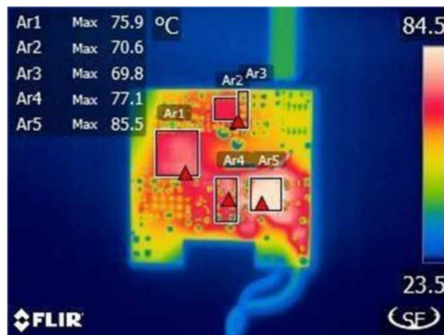
Figure 51 – Bottom Thermal Image, T_{AMB} = 23.5 °C. Ar1: InnoSwitch3-PD, U_1 = 75.9 °C. Ar2: SR FET, Q_2 = 70.6 °C. Ar3: SR FET Snubber = 69.8 °C. Ar4: Primary Snubber = 77.1 °C. Ar5: Bridge Rectifier, BR_1 = 85.5 °C.
