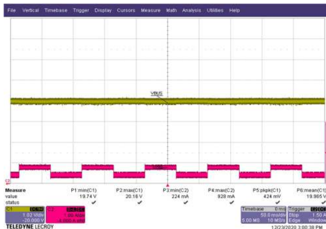
Figure 136 – Transient Response. 90 VAC, 20.0 V, 25% to 50% Load. V_{OUT} = 20.16\text{ V max.}, 19.74\text{ V min.} CH1: V_{OUT} , 1.02 V / div. CH2: I_{OUT} , 1 A / div. Time: 50 ms / div.
