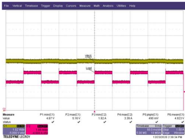
Figure 108 – Transient Response. 90 VAC, 5.0 V, 75% to 100% Load. V_{OUT} = 5.16\text{ V max.}, 4.67\text{ V min.} CH1: V_{OUT} , 1.02 V / div. CH2: I_{OUT} , 1 A / div. Time: 50 ms / div.
