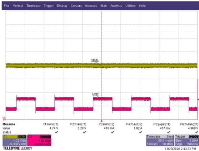
Figure 104 – Transient Response. 90 VAC, 5 V, 25% to 50% Load. V_{OUT} = 5.20\text{ V max.}, 4.74\text{ V min.} CH1: V_{OUT} , 1.02 V / div. CH2: I_{OUT} , 1 A / div. Time: 50 ms / div.
