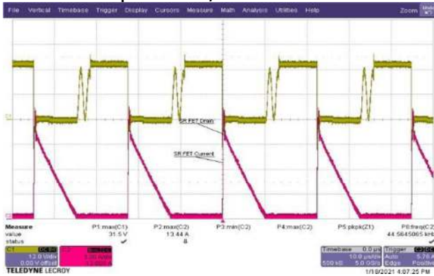
Figure 86 – SR FET Drain Voltage and Current. 90 VAC, 15.0 V, 2 A Load. V_{DS\_SRFET} = 31.5 V Maximum. CH1: V_{DS\_SRFET} , 12 V / div. CH2: I_{DS\_SRFET} , 3 A / div. Time: 10 \mu s / div.
