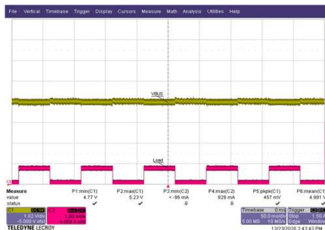
Figure 103 – Transient Response. 265 VAC, 5 V, 0 to 25% Load. V_{OUT} = 5.23 \text{ V max.}, 4.77 \text{ V min.} CH1: V_{OUT} , 1.02 V / div. CH2: I_{OUT} , 1 A / div. Time: 50 ms / div.
