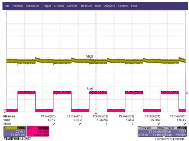
Figure 109 – Transient Response. 265 VAC, 5.0 V, 75% to 100% Load. V_{OUT} = 5.33\text{ V max.}, 4.67\text{ V min.} CH1: V_{OUT} , 1.02 V / div. CH2: I_{OUT} , 1 A / div. Time: 50 ms / div.
