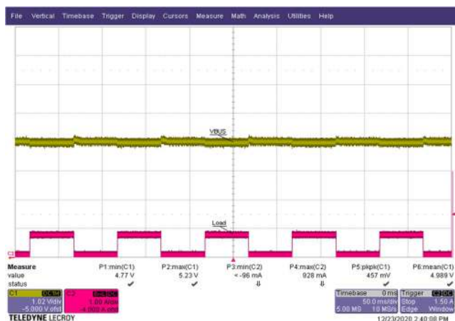
Figure 102 – Transient Response. 90 VAC, 5 V, 0 to 25% Load. V_{OUT} = 5.23 \text{ V max.}, 4.77 \text{ V min.} CH1: V_{OUT} , 1.02 V / div. CH2: I_{OUT} , 1 A / div. Time: 50 ms / div.
