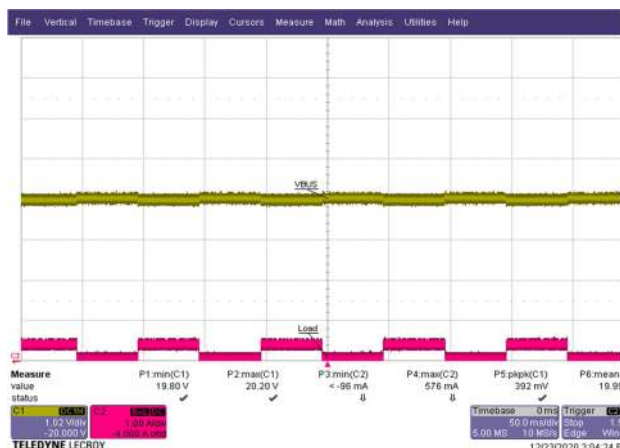
Figure 135 – Transient Response. 265 VAC, 20.0 V, 0 to 25% Load. V_{OUT} = 20.20\text{ V max.}, 19.80\text{ V min.} CH1: V_{OUT} , 1.02 V / div. CH2: I_{OUT} , 1 A / div. Time: 50 ms / div.
