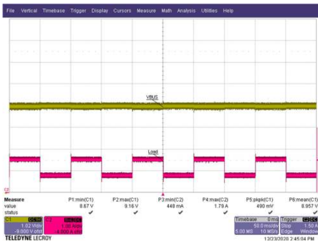
Figure 112 – Transient Response. 90 VAC, 9.0 V, 25% to 50% Load. V_{OUT} = 9.16 \text{ V max.}, 8.67 \text{ V min.} CH1: V_{OUT} , 1.02 V / div. CH2: I_{OUT} , 1 A / div. Time: 50 ms / div.
