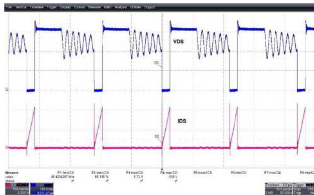
Figure 79 – Primary Drain Voltage and Current. 265 VAC, 15.0 V, 2 A Load. V_{DS\_PRI} = 539 V Maximum. CH1: V_{DS\_PRI} , 150 V / div. CH2: I_{DS\_PRI} , 750 mA / div. Time: 10 \mu s / div.
