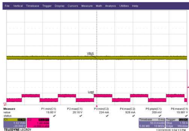
Figure 137 – Transient Response. 265 VAC, 20.0 V, 25% to 50% Load. V_{OUT} = 20.16\text{ V max.}, 19.80\text{ V min.} CH1: V_{OUT} , 1.02 V / div. CH2: I_{OUT} , 1 A / div. Time: 50 ms / div.
