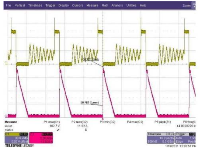
Figure 91 – SR FET Drain Voltage and Current. 265 VAC, 20.0 V, 1.5 A Load. V_{DS\_SRFET} = 103 V Maximum. CH1: V_{DS\_SRFET} , 30 V / div. CH2: I_{DS\_SRFET} , 3 A / div. Time: 10 µs / div.
