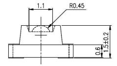
For reflow soldering (propose)
