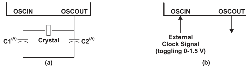
Figure 5-5. Recommended Crystal/Clock Connection
