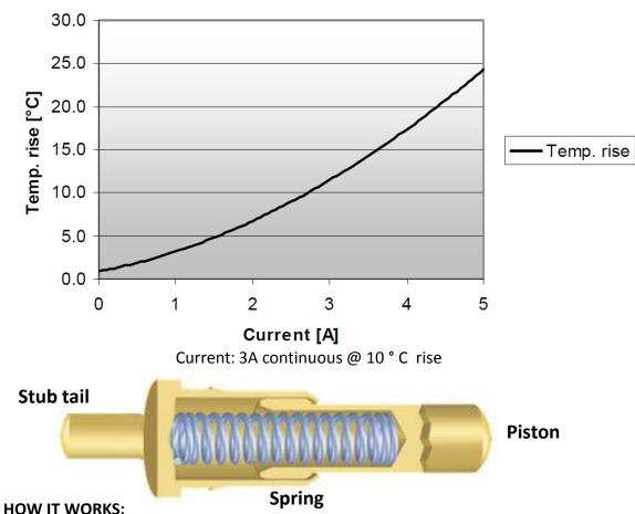
Strong, secure and featuring one piece solid body construction, there are no capped components at the bottom of this spring contact. No seams for solder to wick inside the shell.
