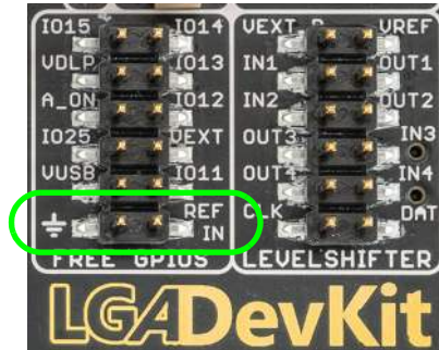
Figure 15: External reference supply and pin header for free level shifter
