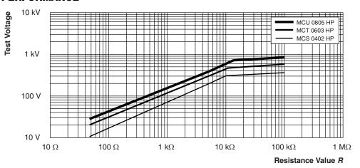
Pulse load rating in accordance with EN 60115-1 clause 4.27; 10  $\mu$ s/700  $\mu$ s; 10 pulses at 1 min intervals; for permissible resistance change  $\pm$  (0.5 % R + 0.05  $\Omega$ )
