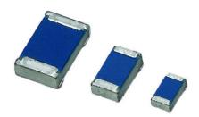
Automotive grade high power MC HP thin film chip resistors are the perfect choice for most fields of modern electronics where high power dissipation, reliability and stability is of major concern. The permissible power rating is specified with up to 400 mW and allows replacement of larger case sizes with next smaller ones. Typical applications include power electronics in automotive and industrial appliances.
