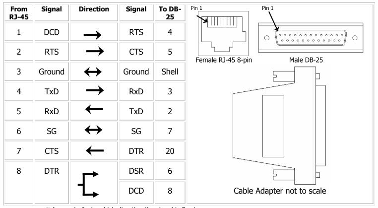
\* Arrows indicate which direction the signal is flowing
