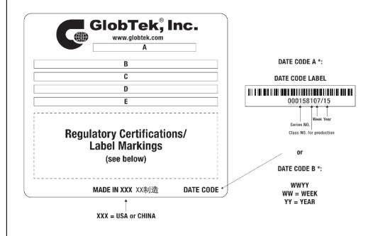
A=DC/DC Switching Power Supply B=P/N: (料号) GTDJ1000USB-F(R6B) C=Model (型号) GTD83050-0505 D=Input (输入)12-24 Vdc, 1A max E=Output (输出)5.0 V == 1.0 A, 5.00W
