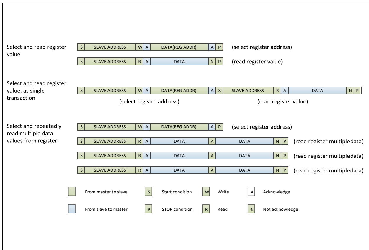
Figure 13: I 2 C Register Read
