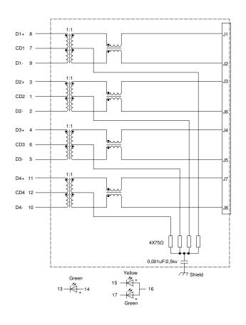
CHECKED REVISION DATE (YYYY-MM-DD) GENERAL TOLERANCE PROJECTION METHOD Œ JefL 001.000 2020-05-12 DIN ISO 2768-1m **S**Vus AI. DESCRIPTION RoHS REACh WE-RJ45 10G Transformer Würth Elektronik eiSos GmbH & Co. KG ORDER CODE EMC & Inductive Solutions Max-Eyth-Str. 1 7499611422 74638 Waldenburg Germany Tel. +49 (0) 79 42 945 - 0 www.we-online.com STATUS BUSINESS UNIT PAGE WÜRTH ELEKTRONIK 2/6 eiSos Valid eiSos@we-online.com
