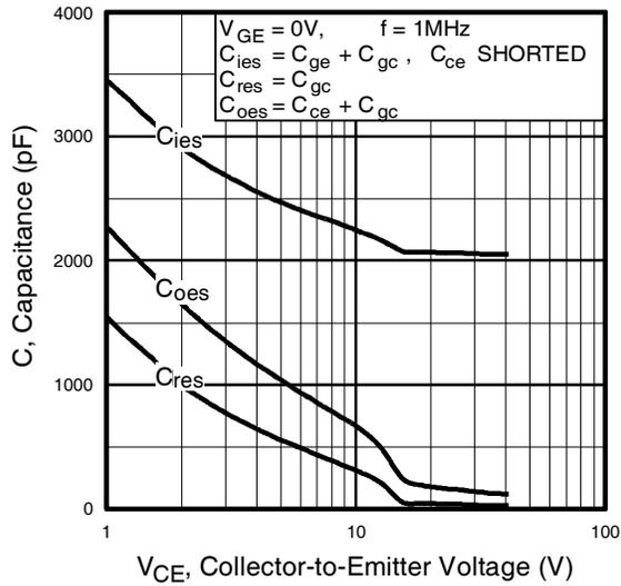
**Fig. 7** - Typical Capacitance vs. Collector-to-Emitter Voltage
