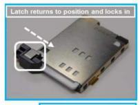
SIM Card is fully inserted
