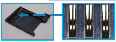
Dual-Point Contacts allow single pin to have different contact forces and lengths to avoid disconnection caused by external vibration's resonance issue
