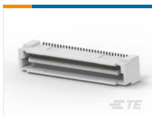
TE Part # CAT-313-PCB60 Free Height Plug Connector: Board-Board, Vertical, 60, 0.8mm
