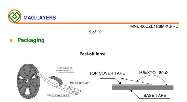
The peel off force of cover tape is 10 to 70 grams in the arrow direction.
