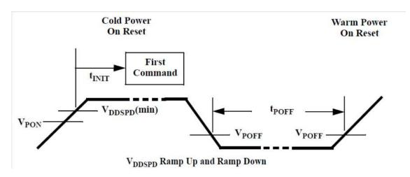
In order to prevent inadvertent Write operations during Power-up, a Power-On Reset (POR) circuit is included. On cold power on,  $V_{DDSPD}$  must rise monotonically between  $V_{PON}$  and  $V_{DDSPD(min)}$  without ringback to ensure proper startup. Once  $V_{DDSPD}$  has passed the  $V_{PON}$  threshold, the device is reset.
