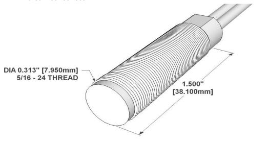
All measurements are in Inches [millimeters]
