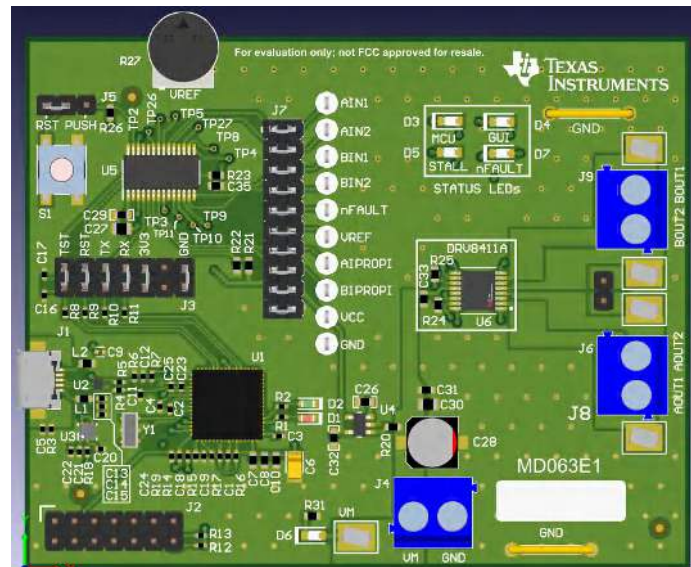
Figure 1-2. MD063 Board for DRV8411AEVM
