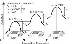
The temperature of the resistor will increase the same △T from the standard terminal part temperature regardlless of the ambient temperature when the same power is applied. This is because there is hardly any heat dissipation from the resistor surface to the ambient air.
