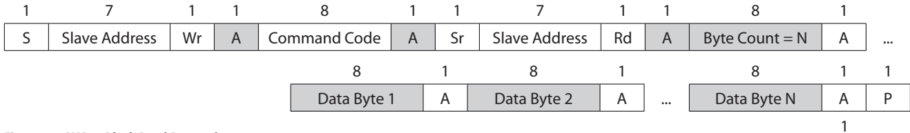
Figure 13. SMBus Block Read Protocol
