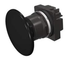
30mm BlackMax, Epoxy Coated Corrosion Resistant Metal Operator, Round Push-Pull Operator Non-Illuminated Mushroom Head Cap Large 2 1/2" (63.5 mm) Plastic, Black 2 Position Maintained, Pull-to-Release UL Listed, CSA Certified NEMA 1,3,3R,4,4X,12,13 & Automotive Standards
