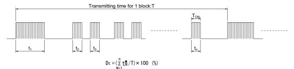
In case the signal format of total duty and/or ON/OFF signal time dosen't meet the conditions noted above, there is a case that reception distance much reduces or output dose not appear.
