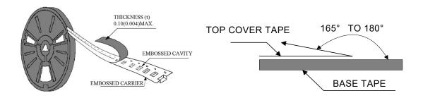
The peel off force of cover tape is 10 to 130 grams in the arrow direction.
