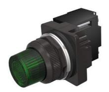
30mm BlackMax, Epoxy Coated Corrosion Resistant Complete Metal Unit Illuminated Indicator Light Full Voltage type, 24V AC/DC Incandescent Lamp, BA9s Glass Lens, Green UL Listed, CSA Certified NEMA 1,3,3R,4,4X,12,13 & Automotive Standards
