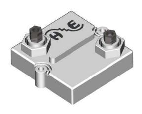
POWER RATING is based on 600 W at 85 °C heat sink temperature. Use of thermal conduction to heat sink is required. Flatness of cooling plate must be better than 0.05 mm overall, and the roughness should not exceed 6.4 um.
