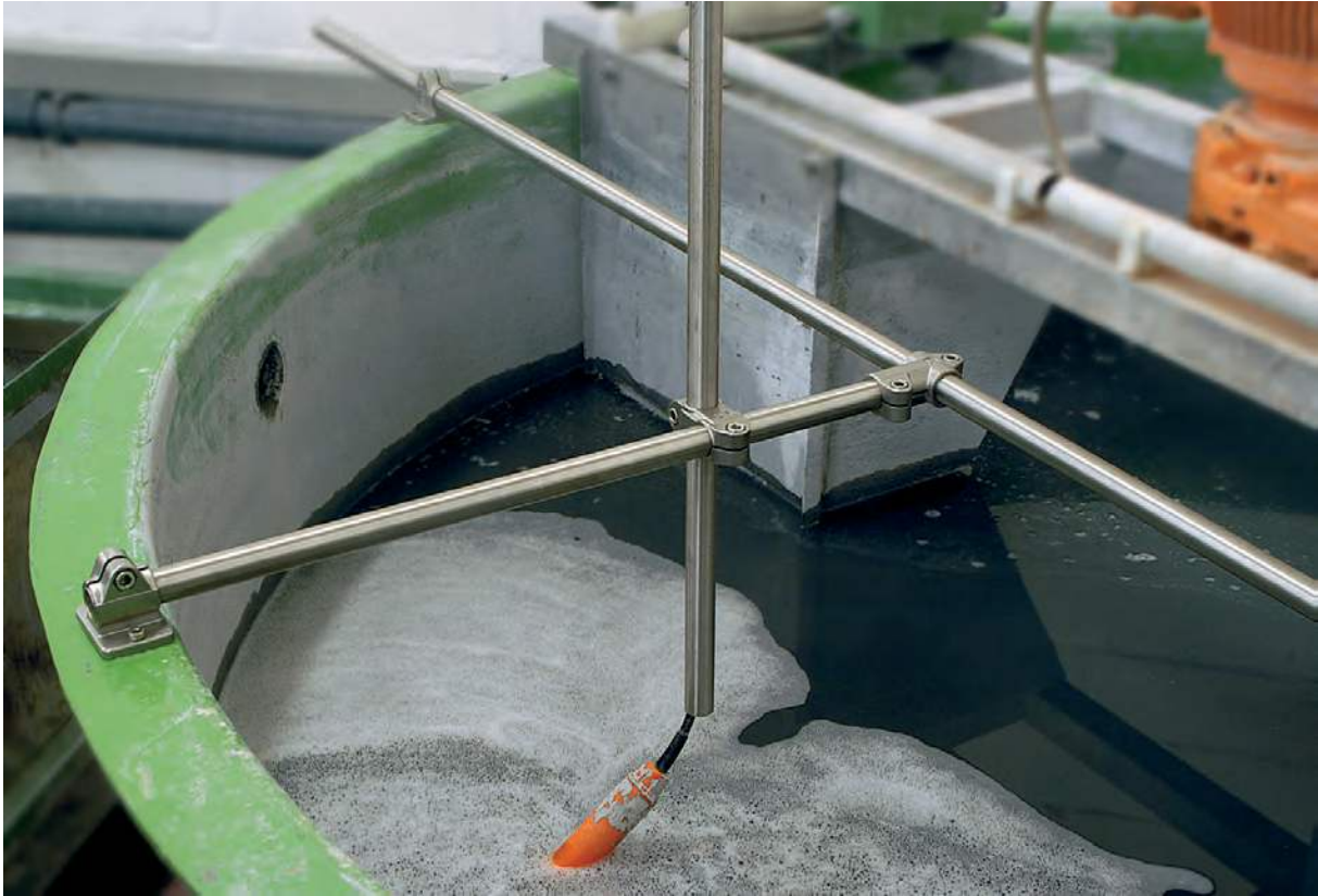
Simple probe fixation in an aggressive environment.
