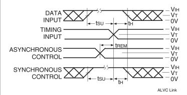
Set-up, Hold, and Release Times
