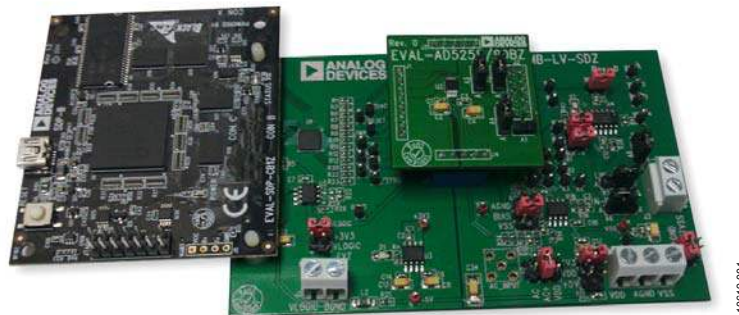
Figure 1. Digital Picture of Evaluation Board with Low Voltage DigiPOT Motherboard and System Demonstration Platform
