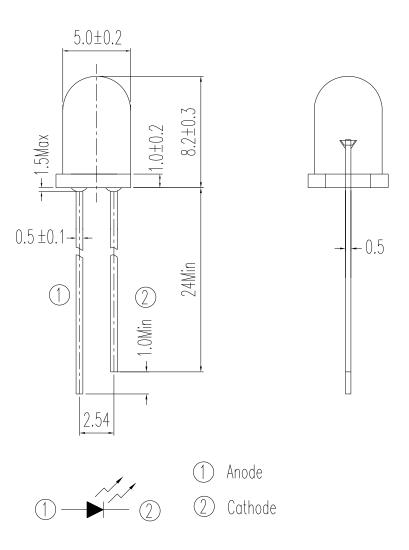
Note: Tolerances unless dimensions ±0.25mm
