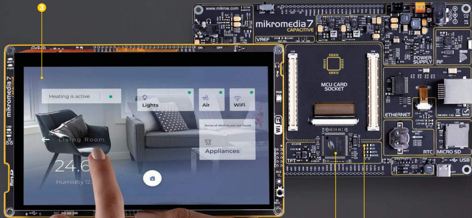
Figure 9: Display and TFT section view
