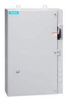
Non-reversing motor starter, Size 2 1/2, Three phase full voltage, Solid-state overload relay, OLRelay amp range 25-100A, 220 240/440 480VAC 60HZ coil, Combination type, 100A non-fusible disconnect, Enclosure NEMA type 4/12, Water/dust tight for outdoors, Standard width enclosure
