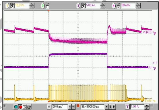
Top: Vo2, CH2 Output Voltage Ripple, (50mV/div) Middle: Io2, CH2 Output Current, (5A/div) Bottom: SWN2, CH2 Switching Node Voltage, (10V/div) Time: 50µs/div
