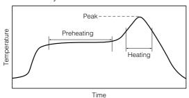
For soldering (Example: Sn/Pb)
