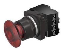
30mm BlackMax, Epoxy Coated Corrosion Resistant Complete Metal Unit Illuminated Twist-to-Release Transformer type, 600V AC LED Lamp Mushroom Head Cap Small 1.79" (45 mm) Plastic Cap, Red 2 Position Maintained, Twist-to-Release with 1 N.O. - 1 N.C. Heavy Duty Contacts, A600/P600 UL Listed, CSA Certified NEMA 1,3,3R,4,4X,12,13 & Automotive Standards
