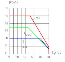
MAXIMUM FORWARD DC CURRENT VS, AMBIENT TEMPERATURE.
