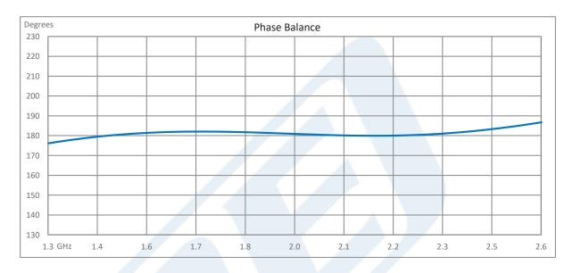
180 Degree SMA Hybrid Coupler from 1.3 GHz to 2.6 GHz Rated to 100 Watts from Pasternack Enterprises has same day shipment for domestic and International orders. Our RF, microwave and millimeter wave products maintain a 99.4% availability and are part of the broadest selection in the industry.
