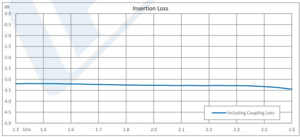
Click the following link (or enter part number in "SEARCH" on website) to obtain additional part information including price, inventory and certifications: 180 Degree SMA Hybrid Coupler from 1.3 GHz to 2.6 GHz Rated to 100 Watts PE2CP1153
