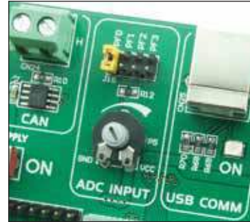
Figure 12-2: Pin PF0 used as input pin for A/D conversion
