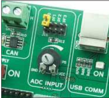
Figure 12-1: ADC (jumper idefault position)
