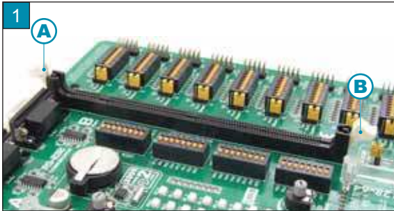
Open extraction levers A and B
