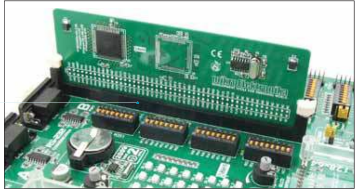
Figure 2-2: DIMM-168P connector with the MCU card inserted
