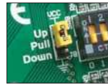
Figure 21-3: J2 in pull-up position
