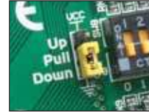
Figure 21-2: J2 in pull-down position
