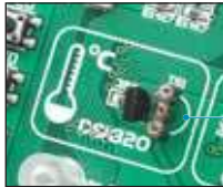
Figure 13-2: DS1820 connector with the DS1820 temperature sensor plugged into
