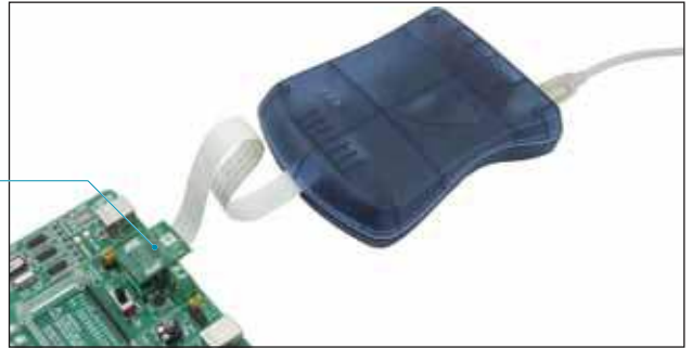
Figure 5-2: JTAGICE mkII connected to the board
