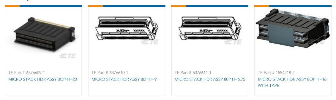
PCB Mount Receptacle, Vertical, Board-to-Board, 80 Position, .6 mm [.023 in] Centerline, Gold, Surface Mount, Signal, Black, Micro Stack
