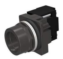
30mm BlackMax, Epoxy Coated Corrosion Resistant Complete Metal Unit Illuminated Push-Pull Operator Transformer type, 120V AC Incandescent Lamp Less Mushroom Head Cap 3 Position Momentary UL Listed, CSA Certified NEMA 1,3,3R,4,4X,12,13 & Automotive Standards
