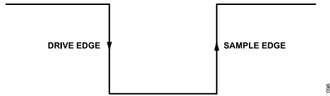
Figure 98. SPI Mode 0 SCLK Edges
