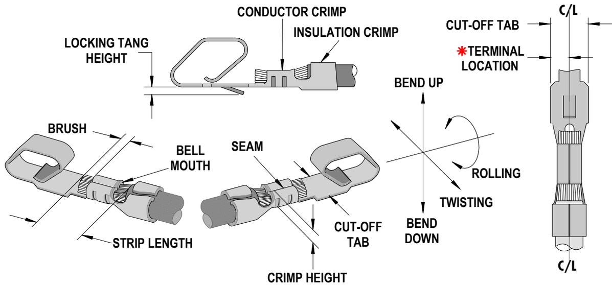
\*Terminal is to be centrally located between the two (2) cut-off edges, within +/- 0.13mm (+/- .005").
