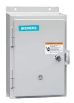
Non-reversing motor starter, Size 1, Three phase full voltage, Solid-state overload relay, OLRelay amp range 0.25-1a, 208VAC 60HZ coil, Non-combination type, Enclosure type 12, Dust/drip proof for indoors, Extra-wide enclosure
