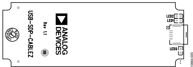
Figure 5. USB-SDP-CABLEZ Board LEDs
