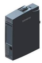
SIMATIC ET 200SP, digital output module, DQ 8x 24VDC/0,5A High Feature, Source output PNP, P-switching, packaging unit: 10 pieces, suitable for BU type A0, color code CC02, channel diagnosis for: short circuit and wire break, power supply, channel failure LED
