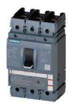
circuit breaker 3VA5 UL frame 250 breaking capacity class H 65kA @ 480 V 3-pole, line protection TM210, FTFM, In=100A overload protection Ir=100A fixed short-circuit protection Ii=10 x In nut keeper kit on both sides
