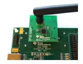
CC2530FM. with the antenna mounted on the SMA connector, can be plugged into a SmartRF05EB. The SmartRF05EB is included in the CC2530 Development Kit [2].
