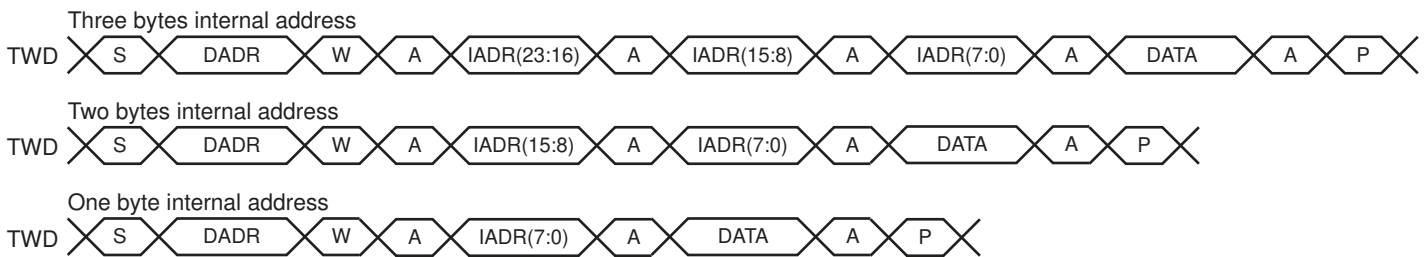
Figure 34-11. Master Write with One, Two or Three Bytes Internal Address and One Data Byte
