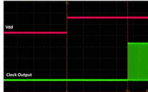
Figure 14. Startup Waveform vs. Vdd
