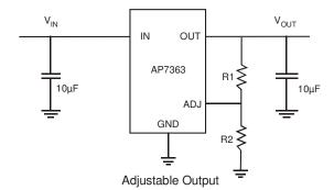
$$V_{OUT} = V_{REF} \Biggl( 1 + \frac{R_1}{R_2} \Biggr) \text{ where } R_2 \leq 10 k\Omega$$
