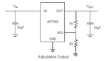
The output voltage is calculated by the following equation:
