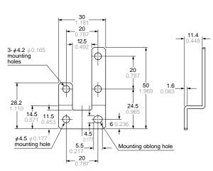
Material: Cold rolled carbon steel (SPCC) (Uni-chrome plated) Two M4 (length 6 mm 0.236 in) pan head screws and two spring washers are attached.
