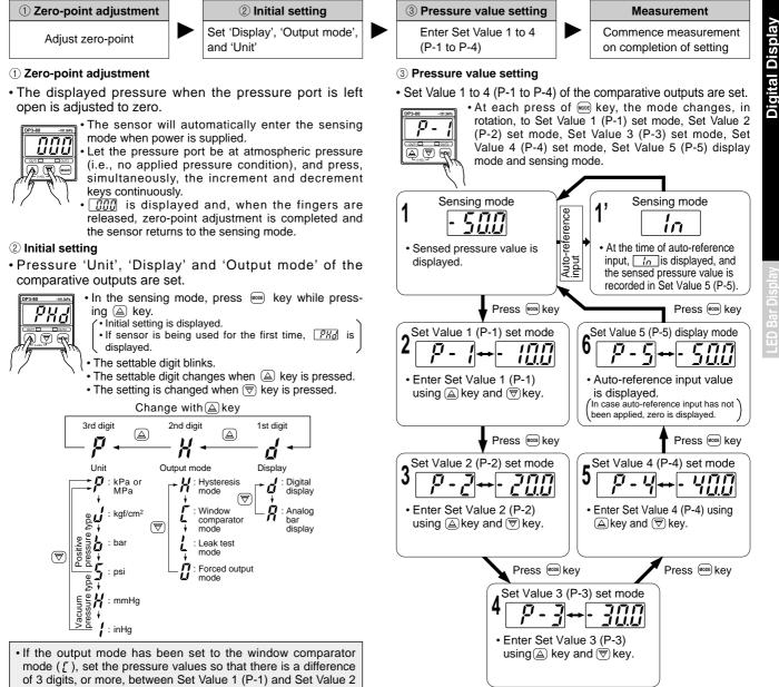
(P-2), and between Set Value 3 (P-3) and Set Value 4 (P-4). Also, if the output mode has been set to the leak test mode ( 1), set the pressure values so that there is a difference of 3 digits, or more, between Set Value 3 (P-3) and Set Value 4 (P-4). However, when unit is set to 'psi' (5), the difference should be 6 digits, or more.
