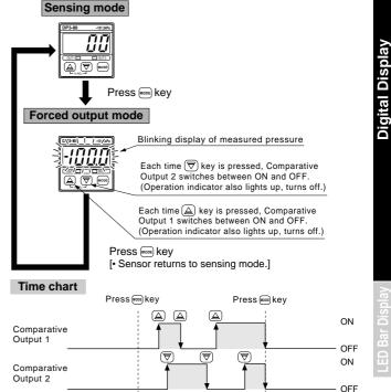
• The comparative outputs are held at the OFF level from the time a change is made to the forced output mode (  $\square$  ) from the other modes.
