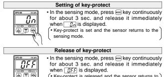
· Key-protect is released and the sensor returns to the sensing mode.
