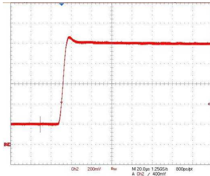
Figure 75. Loop Current Step From 4 mA to 20 mA
